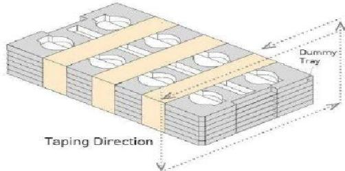
4.2) Tray stacking and taping: Each carton holds **xx** module trays and one empty tray.
